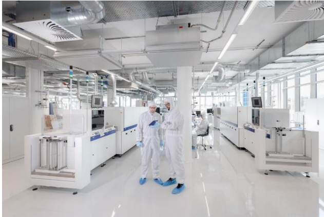
The backend production laboratory of Fraunhofer ISE's PV-TEC photovoltaic technology evaluation center: In this R&D laboratory, production processes for crystalline silicon solar cells are developed and optimized. © Fraunhofer ISE / Photo: Dirk Mahler
